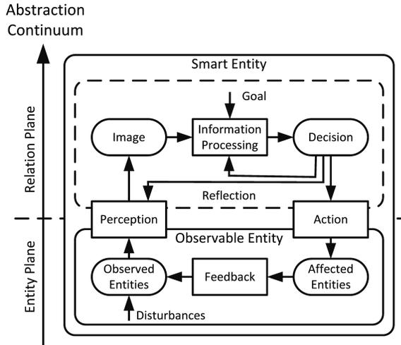
**Figure 4: Perceiving-acting process as a perceptual control loop.**
